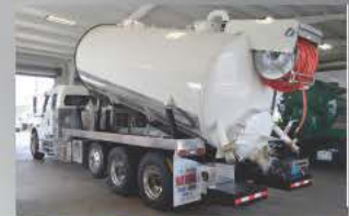
Blower/Jetter Truck 2007 Freightliner M2 475 HP, dump tank 4,800 w/700 Fresh, NVE 900 CFM, 40 GPM Jetter, rear top hydraulic reel, all new equipment.
